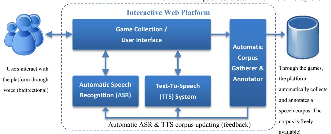
Figure 1 – System architecture
