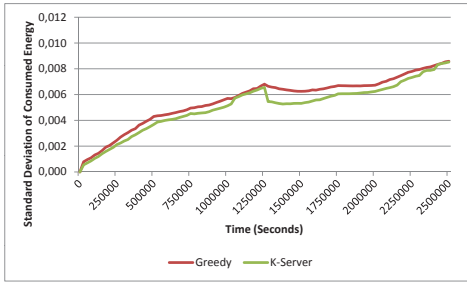
Fig. 7. Standard Deviation of average consumed energy per sensor. Same parameters as in Fig. 6.
