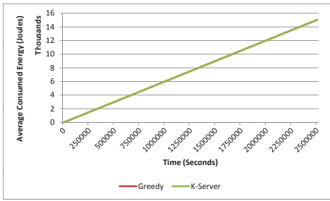
Fig. 6. Average consumed energy per sensor. The side of the event square is 20% of the field side. The number of events per square is 10% of the total number of events.
